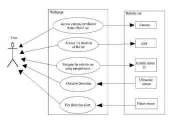
Figure 1: Block Diagram of actual working
